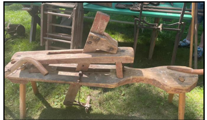
A Shaving Horse for shaping wood into shingles using a draw knife.
